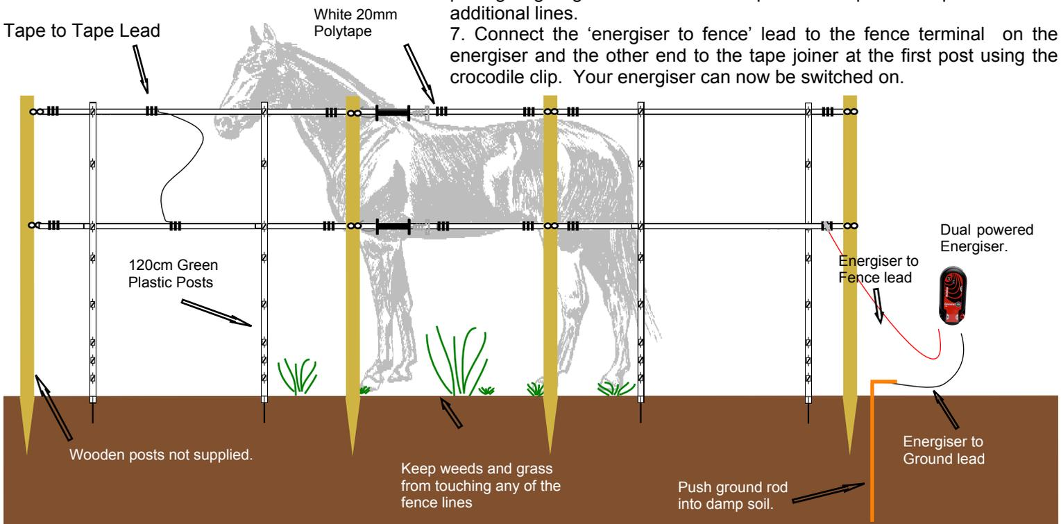
1. Fix your fence energiser to a post or wall or use the stand supplied. Leave switched off until your fence is erected. If using the mains to power the energiser we recommend mounting the energiser undercover or in a building within 25m of your fence. This kit is supplied with a 25m lead out cable which takes the high voltage pulse from the energiser to your fence.
